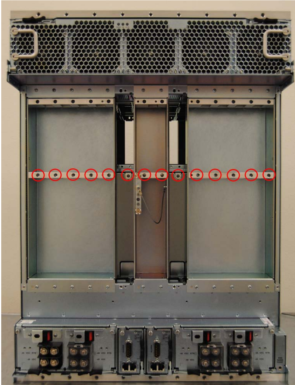
Figure A-3 Recessed Captive Screws in the Ruggedized AXP1440 Shelf
