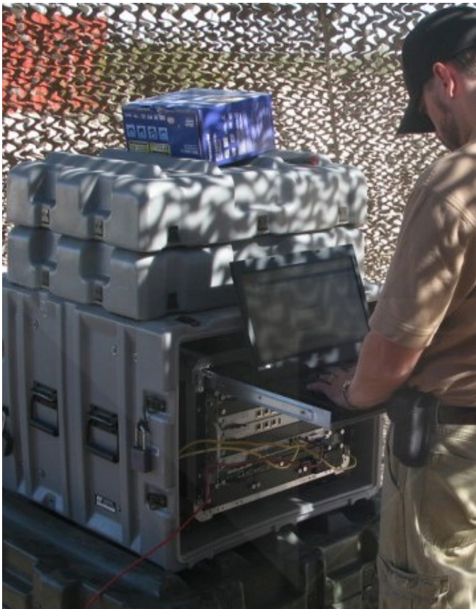
Figure 6: The 6-slot AXP640 chassis used in Computer Systems Center Incorporated® (CSCI) DASCAN. The AXP640 features:
