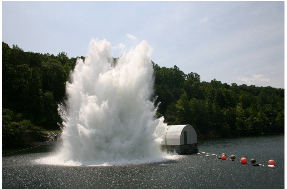
Figure 4: Tests by Northrop Grumman demonstrated that ATCA equipment is able to survive afloat shock testing (commonly called "barge testing"), showing its suitability for deployment as shipboard systems. MIL-S-901D Heavyweight Shock Test Photographs courtesy of National Technical Systems in Rustburg, VA.
